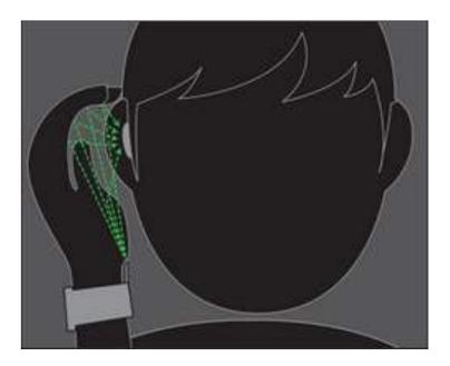
Typical audio is Omni directional. Partial directivity can be given to audio by firing at close range with proper openings. HBand uses normal micro speakers with suitably designed back volume, front volume and opening to provide partial directivity. This method gives partial to full private sound.
